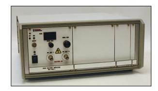
Model HVA-1M Series High Voltage Amplifiers are useful for driving electro-optic Modulators, Pockels cells, Deflectors or Piezoelectric Positioners or Actuators. The driver exhibits high gain, wide frequency response, DC coupled outputs, good stability and can produce an output of 800Vpp (+/-400 Vpk) differential drive into a 100 pF capacity load.
